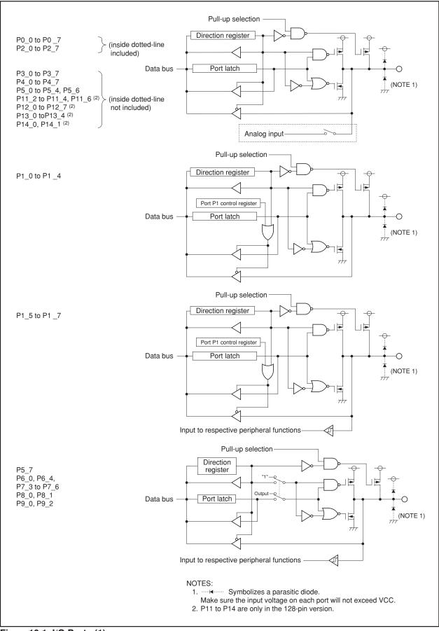
Figure19.1 I/O Ports (1)
